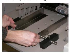
7. When the side guides are adjusted, tighten the screw.
