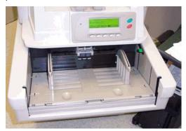
Place the manual feeder on top of the elevator tray using the slots in the manual feeder to align with the side guides. Position the manual feeder to the fully seated position.
