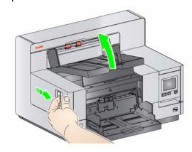
4. Locate the two rails on the left and right side of the transport and slide the manual feed shelf over both of these rails.
