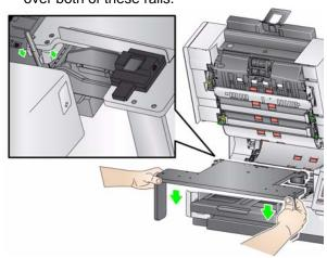
NOTE: Be sure the manual feed shelf has a flat level surface to rest on.
