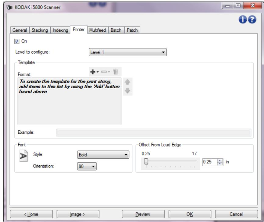
**On** — turns printing on and makes the rest of the options on this tab available.
