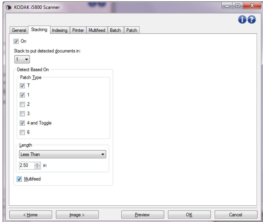
**On** — turns stacking on and makes the rest of the options on this tab available.
