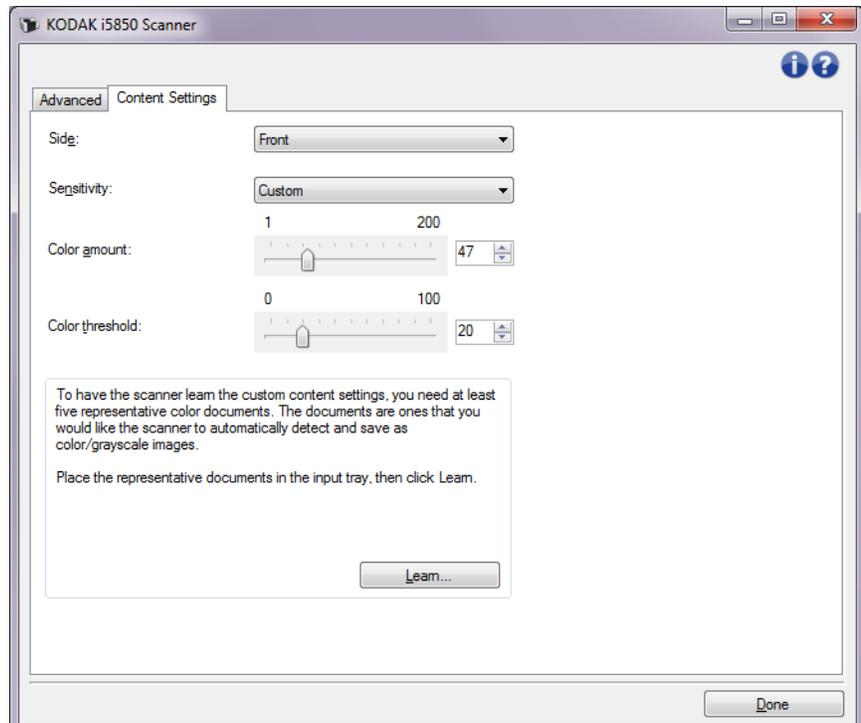
**Side** — determines which side the Sensitivity settings are applied to. This option is only available if **Different settings per side** is checked on the Advanced tab.
