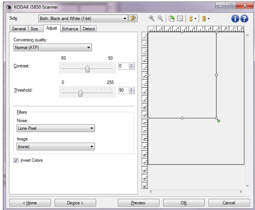
**Conversion quality** — these settings effect how the scanner analyzes a grayscale version of the document which is used to produce the black and white electronic image.
