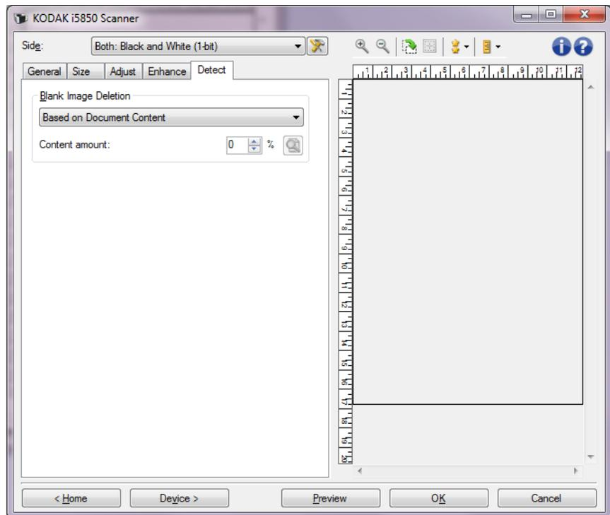
**Blank Image Deletion** — allows you to configure the scanner to not give blank images to the scanning application.
