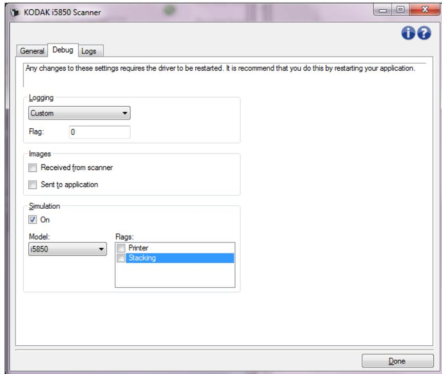
**Logging** — saves the communications between the scanner and a scanning application. The options are: **Off**, **On** or **Custom**.
