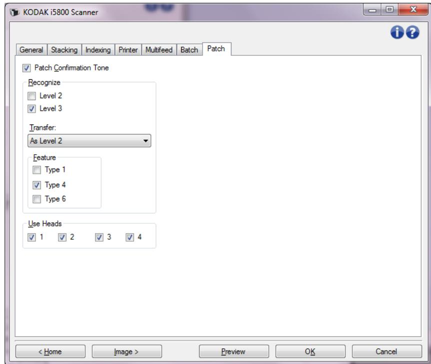
**Patch Confirmation Tone** — the confirmation tone may be used to signal that a patch has been recognized by the scanner. The default is no confirmation tone.
