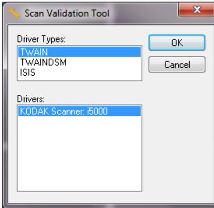
2. Select **TWAIN/TWAINDSM** (or **ISIS**) for the Driver Type and the **Kodak Scanner i15000 Scanner** as the Driver.
