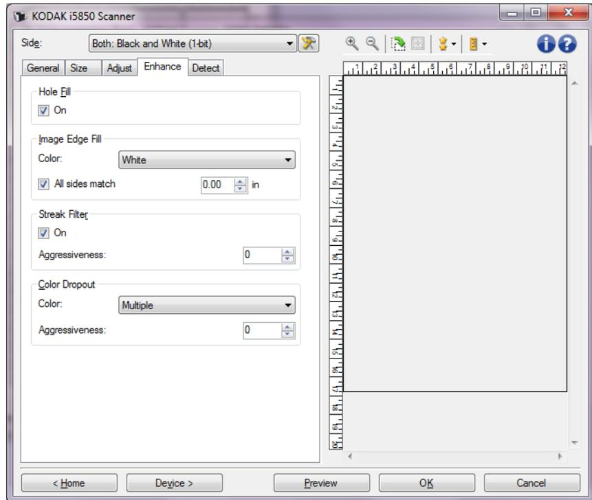
**Hole Fill** —allows you to fill in the holes that are around the edges of your document. The types of holes that are filled include: round, rectangular, and irregularly shaped (e.g. double-punched or those having a slight tear that could have occurred when the document was removed from a binder). Checking **On** turns hole fill on.
