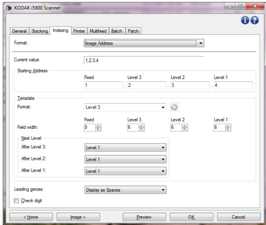
The *Kodak* i5850 Scanner has a new option that was previously not available with scanners having image address capability. The i5850 Scanner allows the scanner drivers to control whether the scanner has Indexing enabled or not. When Indexing is set to **None**, the indexing counters will not be displayed on the Operator Control Panel of the scanner.
