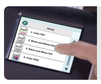
The **Kodak** S2000 Series Scanners allow for up to 20 tasks to be defined. Nine shortcut tasks are predefined but all can be easily customized to fit into your application needs. To add additional tasks to the pre-populated list, select the <NEW> option at the bottom of the Task Shortcut List.
